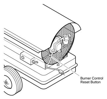
Figure 4 - Burner Control Reset Button
